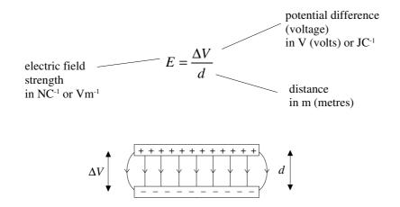
If the potential difference is 1 V, a charge of 1 C would gain 1 J by being pushed through the distance by the field, or 1 J would be required to push the charge through the distance against it.
