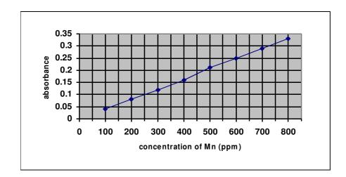
The absorbance reading for a 10 mL sample of manganese ions of unknown concentration is 0.18.
