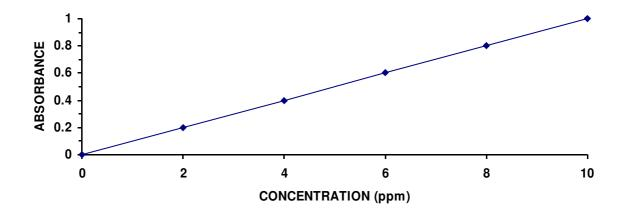
This graph is called a calibration curve and is now used for analysis.
