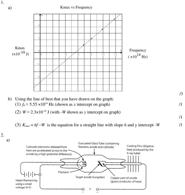
A high potential difference (10 000 - 50 000 V) is used to accelerate electrons across the X-ray tube
