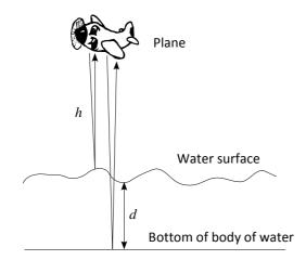
Usually the h beam is an infrared beam fixed pointing directly downwards, and the d beam is a green beam which scans side to side as the aircraft travels, sweeping out the depths of the area it travels over.
