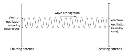
This diagram could be an example of a radio station or television channel transmitter on the left, the wave from which causes the the electrons in the receiving antenna to oscillate, producing a current. The electrons in the receiving antenna will oscillate with the frequency of the wave.
