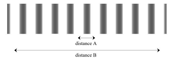
When determining the distance between adjacent maxima, one student measured distance A and found that it was 11 mm. The other student measured distance B and found that it was 91 mm.
