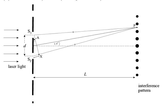
(a) A point P has been marked on the pattern halfway between two of the bright spots. Lines from two of the slits to P have been drawn on the diagram and a point X chosen such that the distance from S1 to P and the distance X to P are equal.
