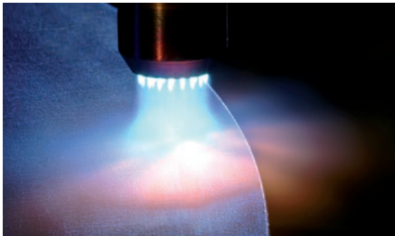
Figure 9. The application of preheat gases.
