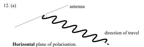
(b) The receiving antenna should be **horizontal**.
