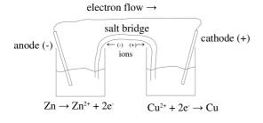
The *salt bridge* (shown labelled) and/or the *electrolyte* (ionic solution): - complete the circuit - allows ions to flow
