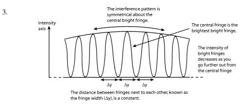
The brighest spots occur when the light has a path difference of  $m\lambda$  therefore constructive. The darkest spots are from a path difference of  $(m+0.5)\lambda$  therefore destructive, and in between are the intermediate path differences.
